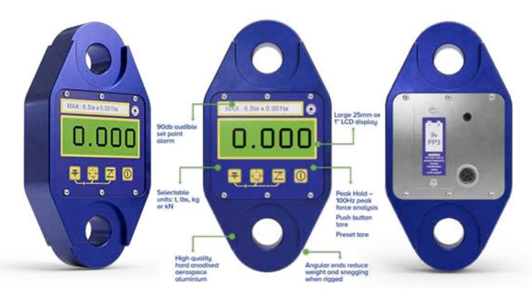
Designed to replace outdated mechanical products still in the field, this 14,300lb (6500kg) Dynamometer, the 'SID', is the latest Crosby SP product to feature their self indicating display.
